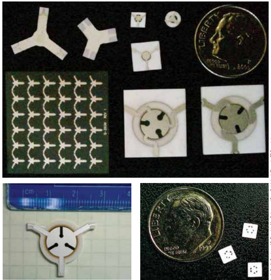
Figure 5. Photographs of integrated cofired mm-wave circulator devices.
